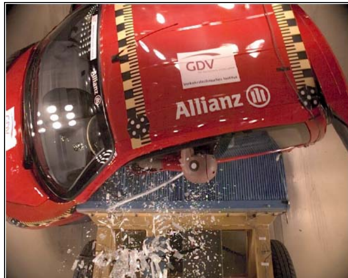
Figure 55: Ligier X-TOO after the lateral crash test [132]
