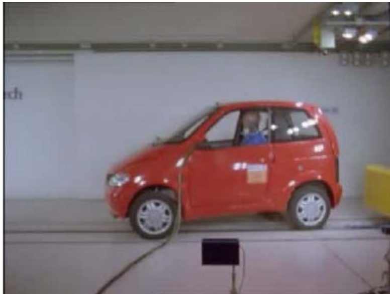
Figure 46: Rear impact test setup [66]
